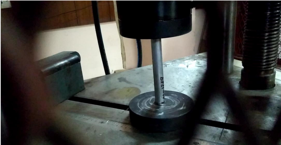
Fig.2. Setup of compressive testing
