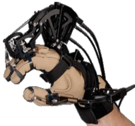
Fig 4: Cyber glove (Haptic Device)
