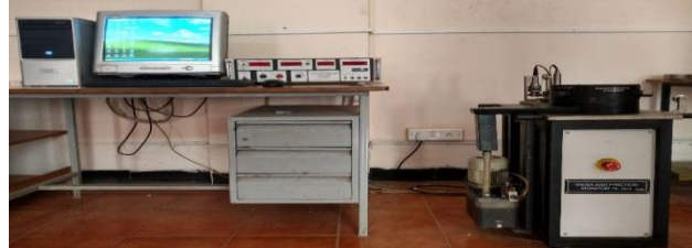
Fig. 2: Pin-on-disc Setup and Wear Monitor
