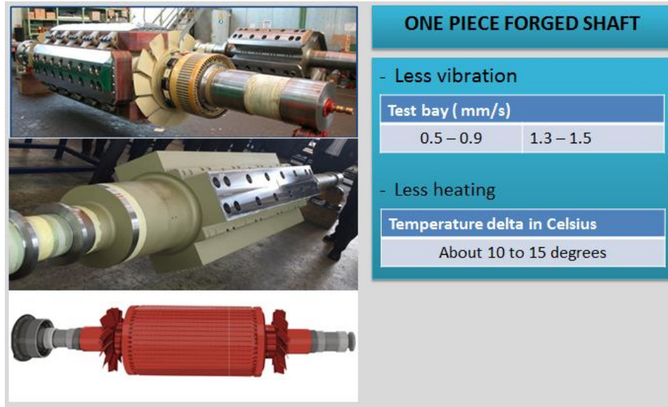
Figure 6: Rotor construction
