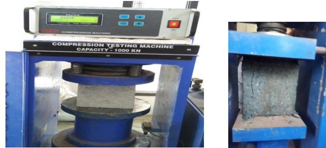
Figure.3 Setup for Compressive strength
